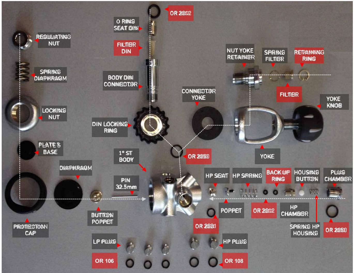
Some important components of the first stage must be replaced during an overhaul. These important components are included in the service kit for first stages 22X (code 46201355 INT/DIN - 46201444 NX) and are highlighted in the **RED FIELDS** above.
