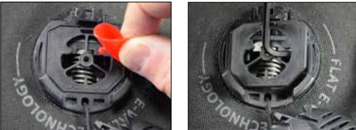
**CAUTION:** Use a small hex key to lift the exhaust plate. Do not pry on the exhaust plate. The plate will be re-used.
