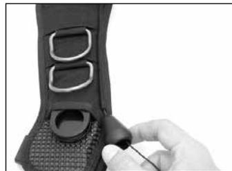
**8** Fold the cord at the 3" (7.6 cm) mark. Tie a double overhand knot as shown. The knot should be 1/2" (1.3 cm) from the 1" (2.5 cm) mark. Pull down on the pull knob so it sits snugly against the knot.
