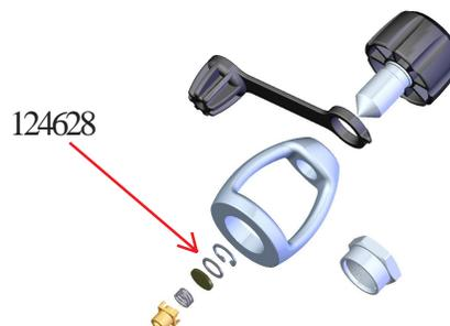
Earlier this year, Aqua Lung began using a brass filter washer, p/n 124628, that has a larger inner diameter. This will allow visual inspection of the filter without the need for disassembly. As regulators come into your stores for service, we would like you to upgrade the filter washer to the new style.
