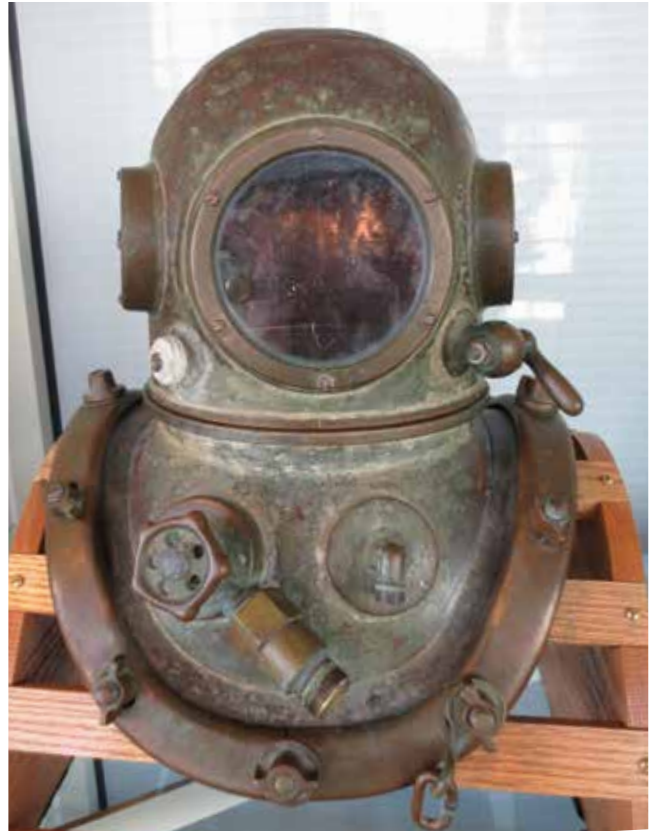
Art McCray style diving helmet with small bonnet on DESCO USN Mark V breastplate. The air control and communications are attached to the front of the breastplate which was a common modification by divers in the Pacific northwest area of the country.
