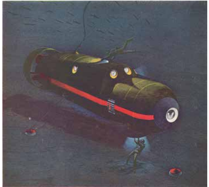
Figure 2: A saturation diver transport vehicle is moored to a location on the seafloor, deploying divers to perform a task. Note the Man-in-the-Sea logo on the forward fuselage.
