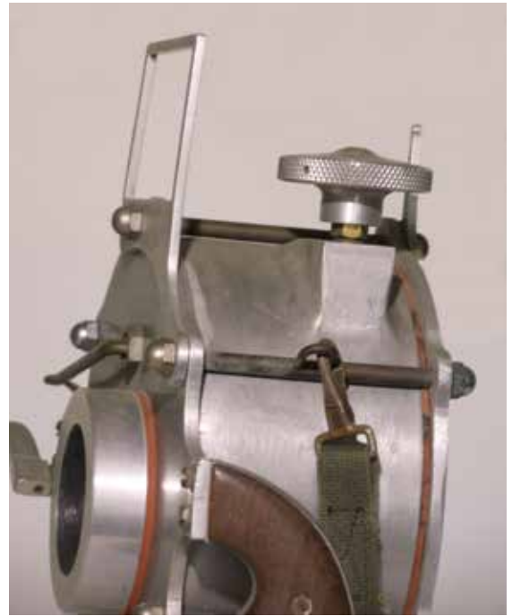
Note the fine work around the film advance knob, the loop for the neckstrap, and the wooden scales on the handle.
