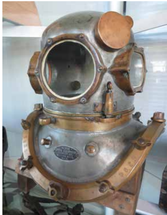
McCray style small volume bonnet helmet serial number 5825 manufactured by Morse Diving Equipment Co. Inc. of Boston, Mass. This helmet does not feature the Hockett breastplate air control valve but shows the scalloped form of the view port frames which was another distinctive feature of Pacific North West helmet design.
